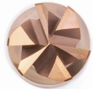
Due to an optimal mix of number of cutting edges, chip breaker and innovative groove shape, the six-edge trochoidal milling cutter OptiMill-Tro-Inox reliably machines workpiece materials from the ISO material group M, which are resistant to high temperatures and tough.
